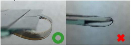
9. Avoid bending the film at IC bonding area. It could damage the IC ILB bonding. It should avoid bending the IC seal area. Please keep the bending distance >1.5mm.
